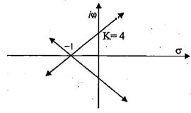
The open-loop transfer function G(s)H(s) of a root locus plot of a system as shown in figure is
