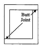
In a core-type single-phase transformer the steel-core is assembled by staggering butt-joints in adjacent layers of laminations vide figures. The purpose served is said to be
