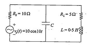
For the circuit as shown, what is the value of C that leads to maximum power transfer to the load, if the value of L is  $0.5 \, \text{H}$ ?
