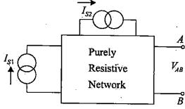
In the network as shown, with  $I_{S1} = 5A$ ,  $I_{S2} = 10A$ ,  $V_{AB} = 120V$ , and with  $I_{S1} = 10A$ ,  $I_{S2} = 5A$ ,  $V_{AB} = 15V$ . What is the value of k to describe  $I_{S1} = k I_{S2}$ , such that  $V_{AB} = 0$ ?
