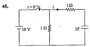
In the circuit as shown in figure, the switch is closed at t=0. The current through the capacitor will decrease exponentially with a time constant of magnitude
