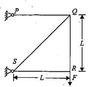
For the truss shown in the figure, the force in the member PQ is
