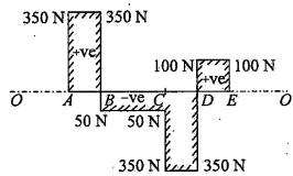
The shear force diagram of a single overhanging beam is shown in figure. One simple support is at end A. The 'total' downward load acting on the beam is
