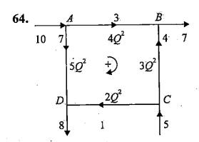
A pipe network is shown with all needful input data to compute the first iteration improved magnitudes of the initially assumed flows in the branches. What will be the such improved flow magnitudes in branches AB and CD? Consider to first decimal accuracy.
