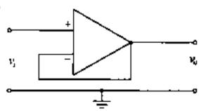
The operational amplifier circuit shown in figure having a voltage gain of unity has
