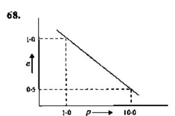
The virgin compression curve with axes adopted as per convention in this regard for a clay soil is shown in the figure. The compression index of the soil is
