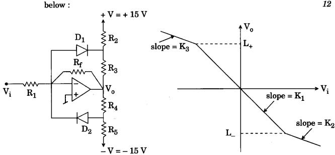
$$(R_1 = 30 \text{ k}\Omega, R_2 = R_5 = 9 \text{ k}\Omega, R_3 = R_4 = 3 \text{ k}\Omega, R_f = 60 \text{ k}\Omega).$$
