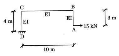
(ii) Use Castigliano's theorem and determine vertical displacement of point C of the beam shown in the figure. Assume E=210 GPa and  $I=150\times10^6$  mm<sup>4</sup>.
