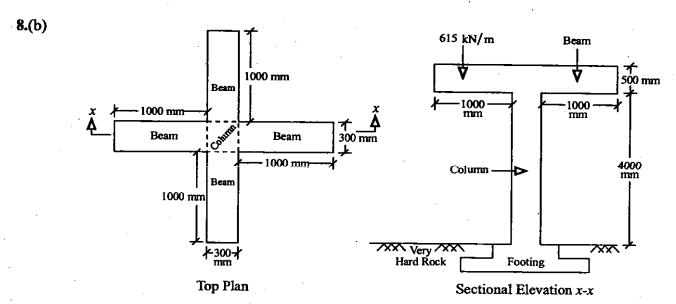
A square column (500 mm  $\times$  500 mm) carries load from two beams, which are mutually perpendicular as shown in figure. Overhang portion of beams carry a total load of 615·0 kN/m (include self-weight). Design the column at top of footing level. Footing is fully embedded in very hard rock. Beams are restrained against rotation at Beam-column junction. The minimum eccentricity is less than 0·05 times the lateral dimension of column. Sketch all details required at column cross-section.
