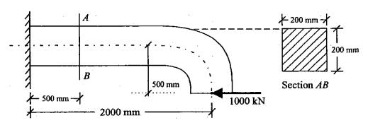
A bracket has been loaded as shown in figure. Compute the top and bottom fibre stress at section A-B.
