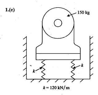
A motor of 150 kg mass is supported by four springs as shown in figure. Each of the springs has a stiffness of 120 kN/m. The unbalance of the rotor is equivalent to a mass of 40 g located at 150 mm from the axis of rotation. The motor is constrained to move vertically. Find
