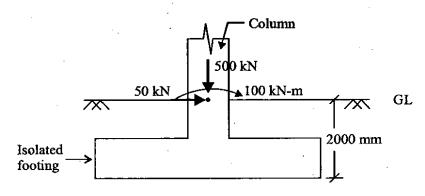
An isolated footing is transferring load from a column (300 mm × 300 mm) as shown in figure. Arrange the plan dimensions of footing so that there will be uniform soil pressure intensity. Following parameters may be used.
