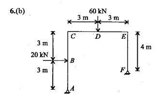
Find the collapse load for a frame of uniform cross-section shown in figure under the applied forces. Also determine the minimum section in steel required to resist the applied forces. 20
