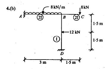
Analyse the frame shown in figure by slope deflection method and draw the B.M.D. and S.F.D. 20
