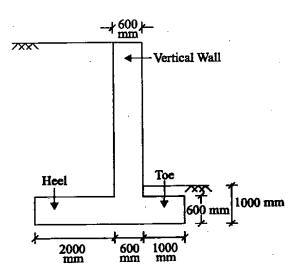
Design and sketch the reinforcement in vertical wall, Toe slab and Heel slab (for maximum Bending moment and maximum shear force only) for the cantilever retaining structure shown in figure. Following parameters may be used for design and sketch:
