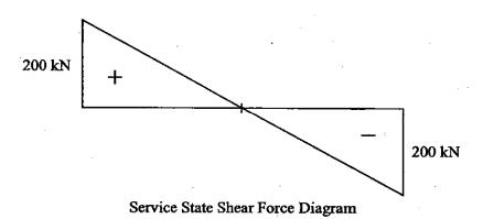
Design the reinforcement at critical section only for a beam for which Bending moment and shear force diagram has been shown in figure. Following parameter may be used for design:
