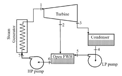
Specific enthalpy of steam at location 2 is 2624 kJ/kg, specific enthalpy of water at location 5 is 226.7 kJ/kg and specific enthalpy of saturated water at location 6 is 708.6 kJ/kg. If the mass flow rate of water entering the open feed water heater (at location 5) is 100 kg/s then the mass flow rate of steam at location 2 will be \_\_\_\_\_\_ kg/s (round off to one decimal place).
