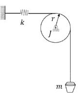
The pulley radius is r and its mass moment of inertia is J. Assume that the mass is vibrating harmonically about its static equilibrium position. The natural frequency of the system is
