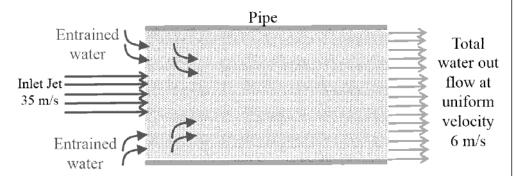
The flow rate of entrained water is \_\_\_\_\_\_ litres/s (round off to two decimal places).
