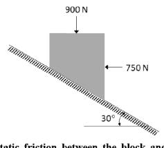
The coefficient of static friction between the block and surface is \_\_\_\_\_\_ (round off to two decimal places).
