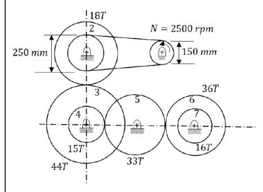
Diameters of pulleys of belt drive and number of teeth (T) on the gears 2 to 7 are indicated in the figure. The speed and direction of rotation of gear 7, respectively, are
