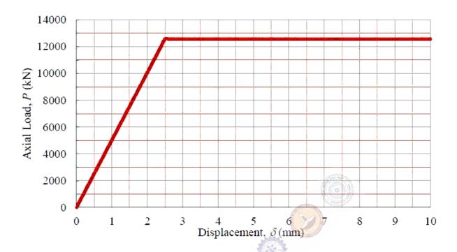
Assume the yield stress of steel as 250 MPa. The complementary strain energy (in N-mm) stored in the bar up to its linear elastic behavior will be
