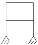
If the axial and shear deformations in different members of the frame are assumed to be negligible, the reduction in the degree of kinematical indeterminacy would be equal to
