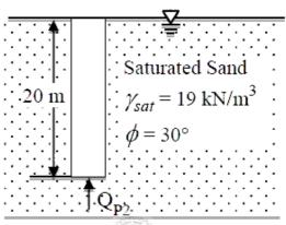
If  $Q_{p_1}$  and  $Q_{p_2}$  represent the ultimate point bearing resistances of the piles under dry and submerged conditions, respectively, which one of the following statements is correct?
