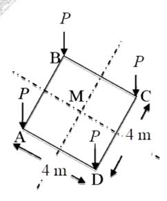
The vertical stress increment (in kPa, up to one decimal place) due to these loads according to the Boussinesq's equation, at a point 5 m right below M, is \_\_\_\_\_
