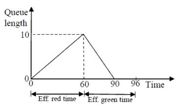
At time t = 0, the light has just turned red. The effective green time is 36 seconds, during which vehicles discharge at the saturation flow rate, s (in vph). Vehicles arrive at a uniform rate, v (in vph), throughout the cycle. Which one of the following statements is TRUE?
