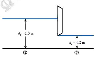
It is observed that the depth of flow is 1.0 m upstream of the gate, while the depth is 0.2 m downstream of the gate. Assuming a smooth flow transition across the sluice gate, i.e., without any energy loss, and the acceleration due to gravity as 10 m/s<sup>2</sup>, the discharge (in m<sup>3</sup>/s, up to two decimal places) passing under the sluice gate is
